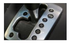
The "park to reverse" or "false park" defect is a flaw in a vehicle's transmission in which it appears that the vehicle is in park. However, the transmission is neither in park nor in hydraulic reverse. Instead, it is in an unstable position between the two gears. Slight movements can cause the vehicle to self-shift into reverse.
