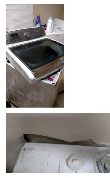
e. ... The entire top of the unit separated and flew across the room exploding that [sic] glass across the laundry room and into our hallway, and the explosion put holes in the wall, damaged shelves, etc. If my wife or son were in the room when this happened, I have no doubt that they would be in the hospital or possibly even killed. (Report date: November 18, 2015; Model No.: WA50F9A6DSW/A2; Photographs Below)
